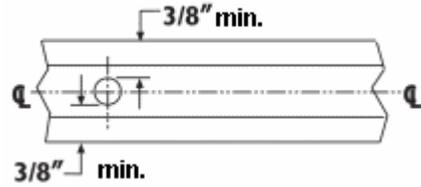
When a hole is on the centerline of the width of a heater the maximum hole size can be determined by subtracting 3/4" from the heater width.
